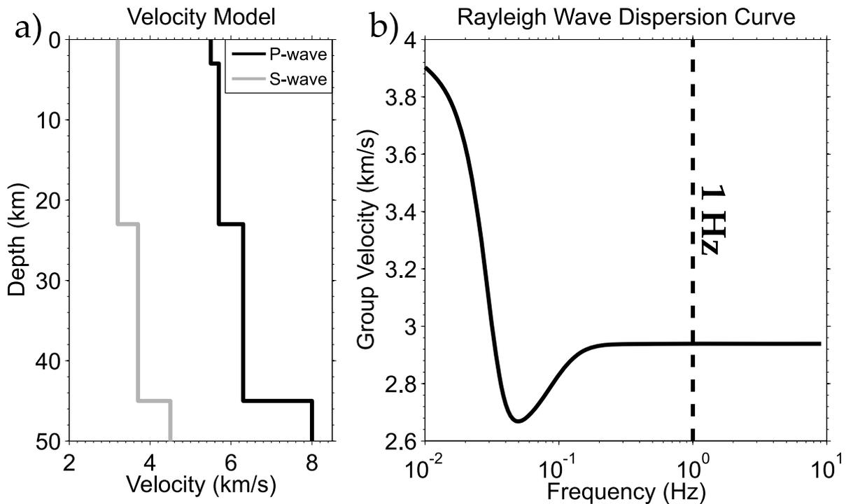
**Figure 7.** (a) Velocity structure of the Himalayas of Nepal determined by Monsalve *et al.* (2006). *P*- and *S*-wave velocities are illustrated by the black and grey lines, respectively. (b) Rayleigh wave dispersion curve for the given model in (a). Note that for the frequencies of interest ( $>1$  Hz), the group velocity of surface wave is constant with a value of  $2.9\text{--}3\text{ km s}^{-1}$ .
