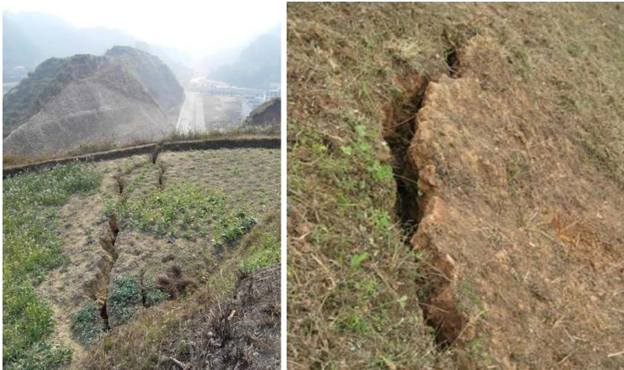
Fig. 7. In-site observation of surface cracks at the top of a slope.
