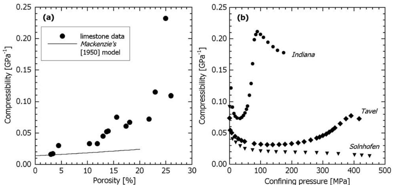
**Figure 2.** (a) Compilation of compressibility data on limestones. Model curve shows Mackenzie's [1950] model prediction of the compressibility based on equation (1) in the text. (b) Compressibility data of three limestones as functions of confining pressure.
