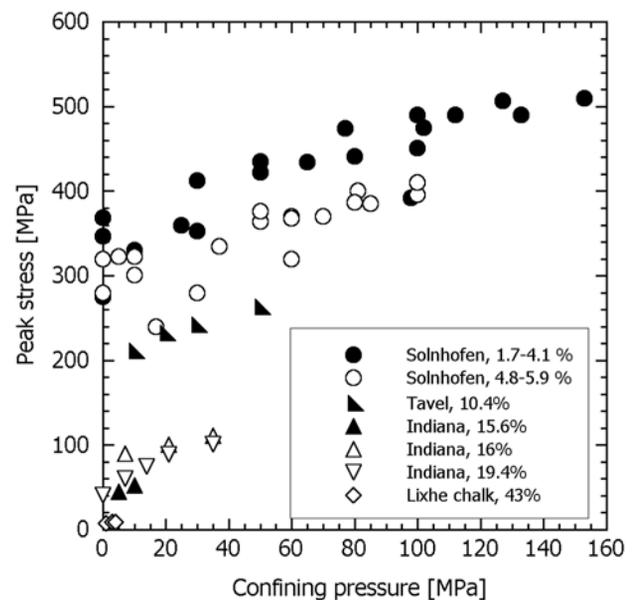
**Figure 10.** Compilation of peak stress data for carbonate rocks of different porosities. (Initial porosity in per cent is indicated for each rock.) Data sources: Solnhofen limestone: compilation in *Baud et al.* [2000]; Tavel limestone, 10.4%: this study; Indiana limestone, 15.6%: this study; Indiana limestone, 16.0%: *Boozer et al.* [1962]; Indiana limestone, 19.4%: *Schwartz* [1964]; Lixhe chalk: *Homand and Shao* [2000].
