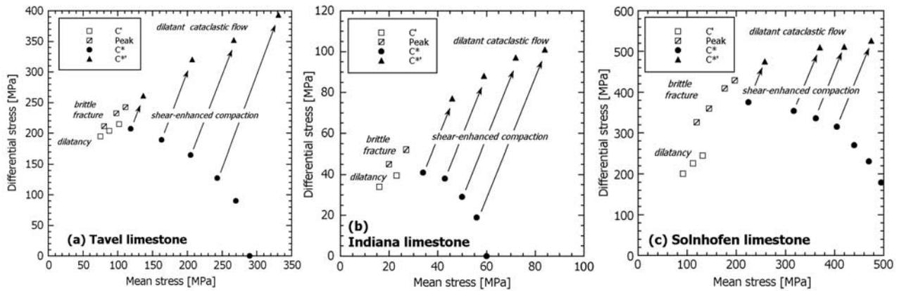
**Figure 8.** Stress states  $C$ ,  $C^*$  and  $C^{*/'}$  and peak stress are shown in the stress space for (a) Tavel (b) Indiana, and (c) Solnhofen limestone. Three regimes of inelastic failure can be identified: brittle fracture, dilatant cataclastic flow, and shear-enhanced compaction.
