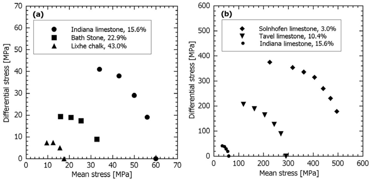
**Figure 11.** Compilation of compactive cataclastic flow yield envelopes for carbonate rocks of (a) high and (b) low porosities. For reference, Indiana limestone appears in both graphs. Initial porosity in per cent is indicated for each rock. Data sources: Lixhe chalk: *Homand and Shao* [2000]; Bath Stone: *Elliot and Brown* [1986]; Indiana limestone: this study; Tavel limestone: this study; Solnhofen limestone: *Baud et al.* [2000].
