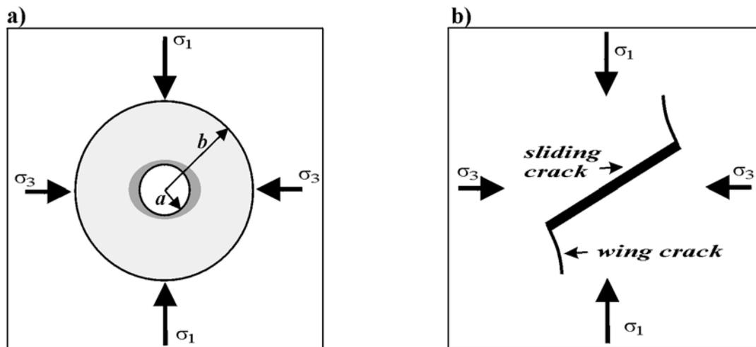
**Figure 6.** Two conceptual models of failure micromechanisms. (a) Plastic collapse of an isolated spherical pore may account for inelastic compaction. Dark-gray zone represents the initiation of plastic deformation while the remaining volume (light-gray) experiences elastic deformation. (b) Dilatancy and brittle faulting were explored by wing crack model.
