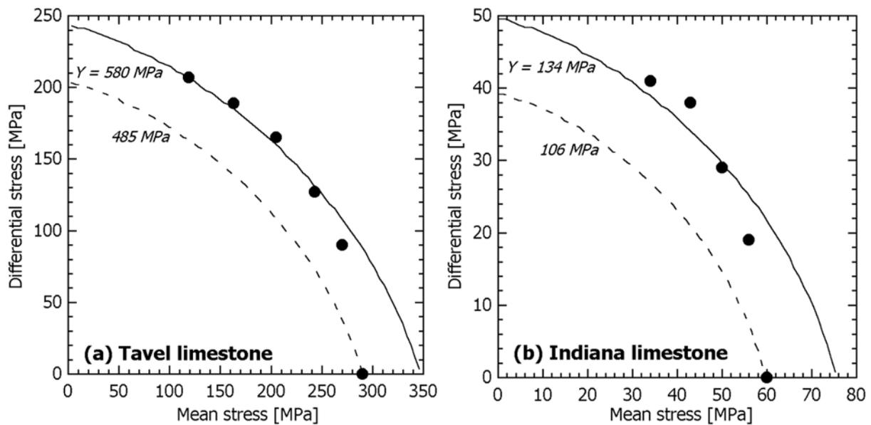
**Figure 12.** Initial yield envelopes for (a) Tavel and (b) Indiana limestone assuming matrix material governed by von Mises yield criterion calculated using the model of *Curran and Carroll* [1979]. The solid points represent  $C^*$  data outlining the cataclastic flow envelope, solid curve represents the best fit to the  $C^*$  data and dashed curve the fit of solely the pore collapse pressure  $P^*$ . The yield stress  $Y$  corresponding to each of the curves is indicated.
