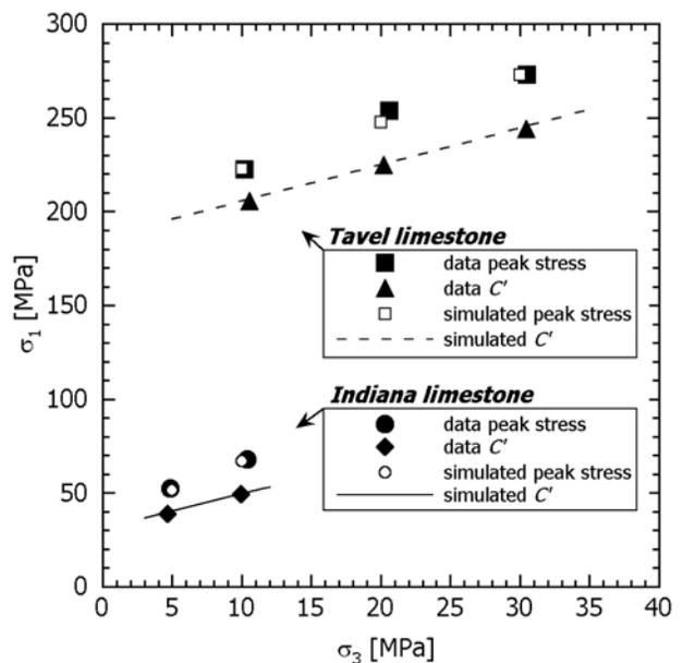
**Figure 9.** Comparison of the experimental data on brittle faulting (onset of dilatancy  $C'$  and the peak stress) for Indiana and Tavel limestones with predictions based on wing crack model. The relevant parameters are compiled in Table 3. Equations (2) and (3) of Baud et al. [2000] were used to fit the onset of dilatancy  $C'$  and the peak stress, respectively.
