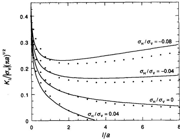
Fig. 4. Normalized stress intensity factor  $K_I$  as a function of wing crack length  $l$  for indicated  $\sigma_H/\sigma_V$  with  $\mu = 0.3$  and  $\beta = 45^\circ$ . Solid lines are from the analytic estimate (8) and symbols are for the exact numerical calculation [5].
