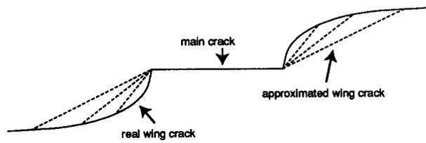
Fig. 2. The real wing crack is replaced by a straight one the orientation of which  $\theta$  depends on its length.
