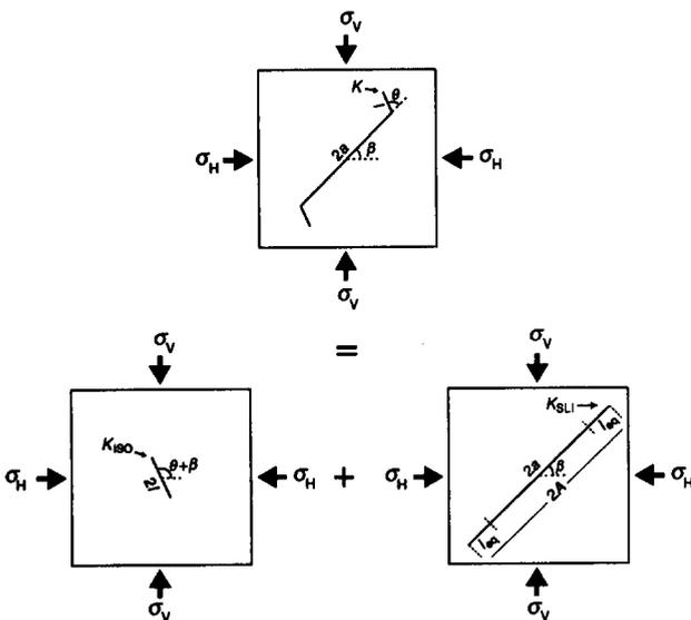
Fig. 3. A superposition technique is used to calculate an approximate  $K_I$  value for the straight wing crack. The signification of  $l_{eq}$  and  $A$  is given in the text.
