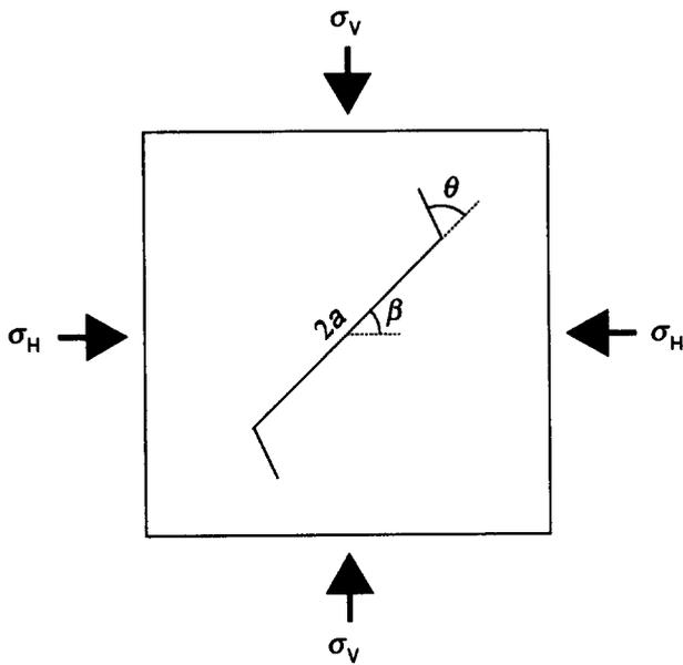
Fig. 1. Sketch illustrating the propagation geometry of a sliding crack under compression.
