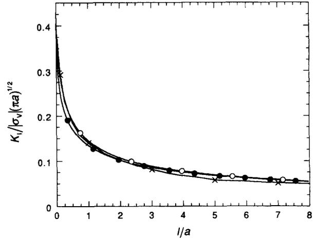
Fig. 5. Normalized stress intensity factor  $K_I$  as a function of wing crack length  $l$  for a main sliding crack lying at  $\beta = 45^\circ$  and subjected to uniaxial compression ( $\mu = 0.3$ ). Comparison between the derivation by Horii and Nemat-Nasser [14] [equation (9), open symbols] and the present derivation [equation (8), closed symbols]. The exact results by Horii and Nemat-Nasser [5] are given for reference ( $\times$ -symbols).
