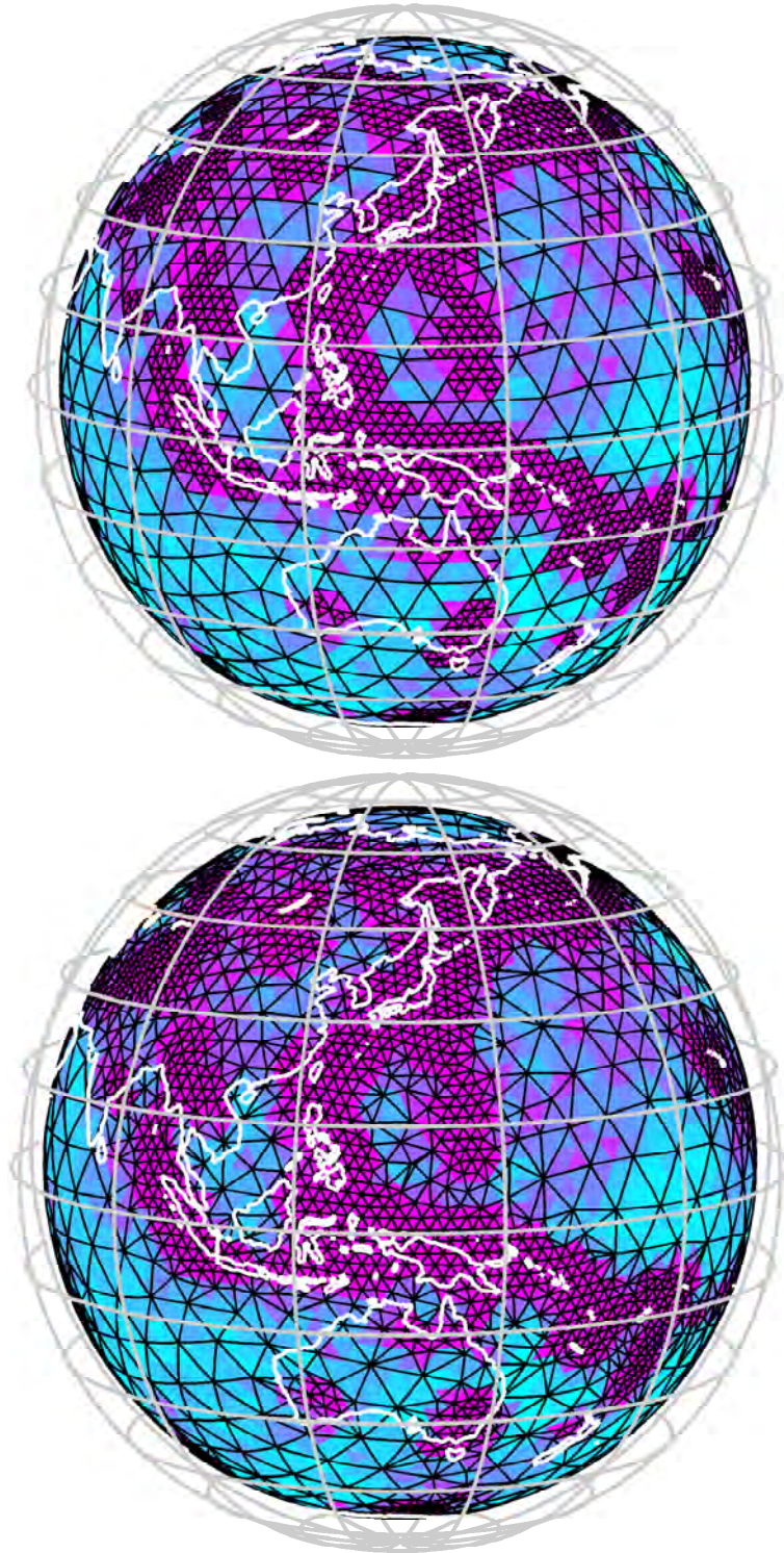
Figure 3.7: Starting (upper frame) and optimized (lower frame) grids, displayed in black, of the sixth layer (530–660 km depth). The resolution length function, \ell(\mathbf{r}) , is superimposed, with a linear colorscale ranging from 210 km (in cyan) to 850 km (in magenta).
