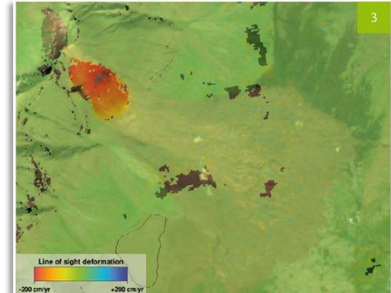
Figure 3. Yearly rate map of the Fagraskógarfjall landslide between July and November 2017. Green represents relatively stable areas while the red-yellow region highlights significant slip of the landslide. Up to 2 m per year of slip may have occurred in some parts of the landslide. © CGG 2018. Images contain modified Copernicus Sentinel data (2018).
