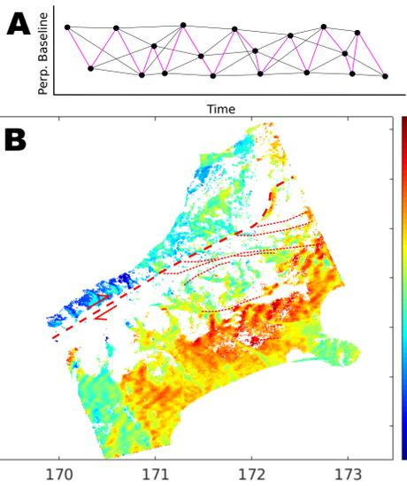
Fig 1) (A) 33 sequential 12-day interferograms (purple lines) of track 125A were taken from a network produced with the LiCSAR processor and chained together to provide total cumulative displacement over 2017. (B) This results in a loss of signal near to the AF (thick dashed line), as well as larger LOS displacements from coast-to-coast than would be expected- in the near field the high incidence angle means only approximately half (~20 mm/yr) of displacement should be resolved in LOS.
